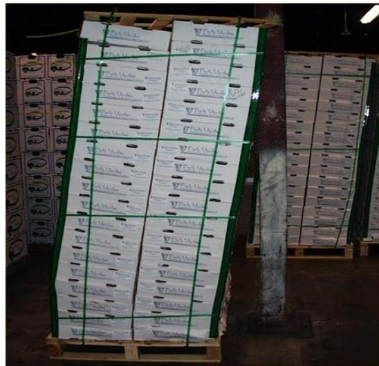
Pallets that are bound by straps can be under a lot of tension and may snap like a whip when cut. This has potential for cuts, bruises and eye injuries and can be particularly dangerous when steel straps are being cut. Operators should wear gloves and use eye protection when appropriate.
